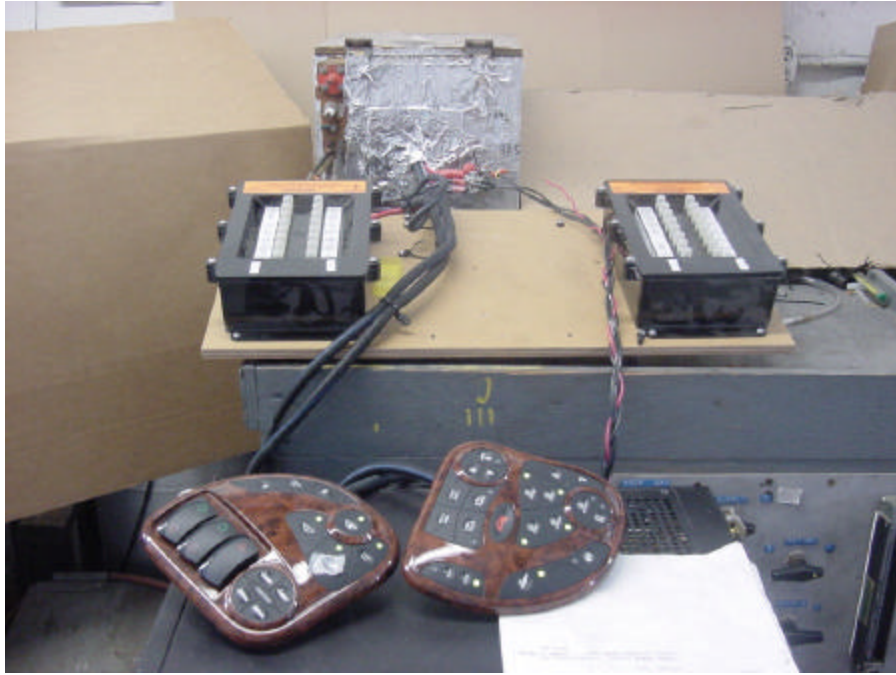
Figure 3 View of set-up with dummy loads attached.
