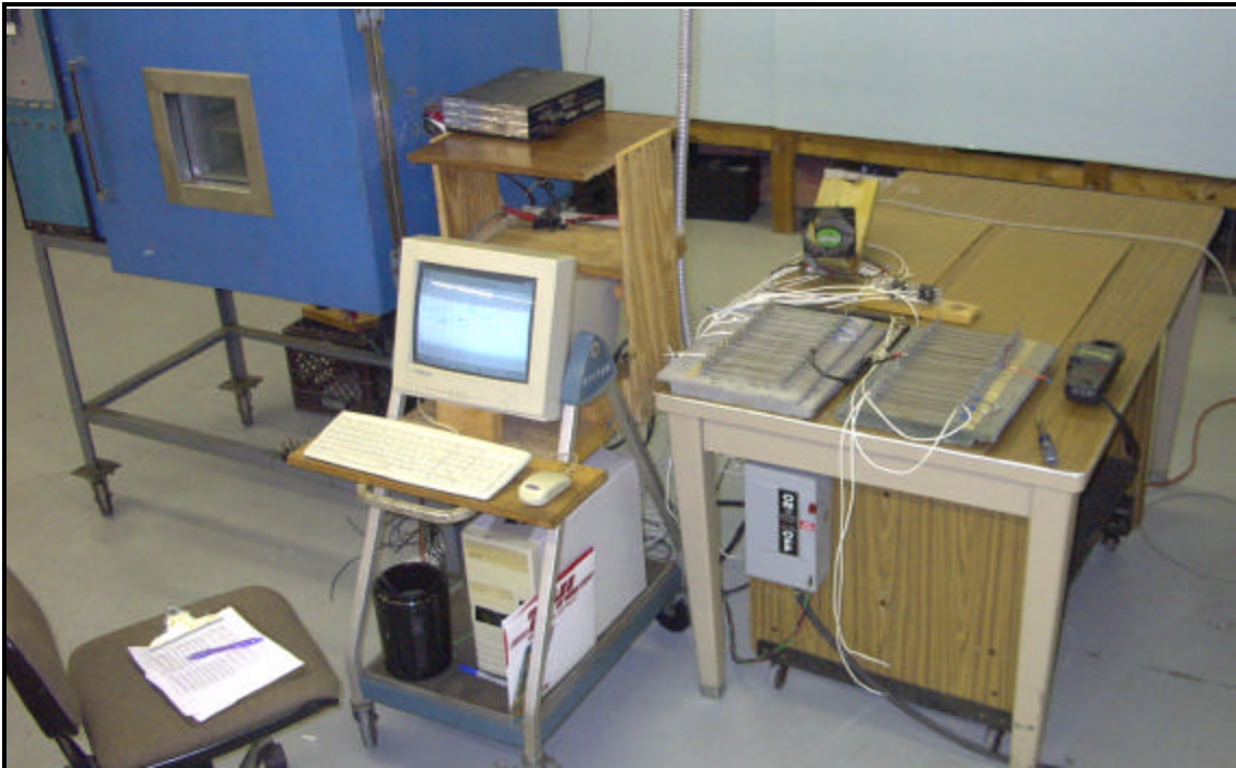
Overall view of test setup. Data acquisition unit position directly opposite temp. chamber's access port.
