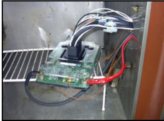
Typical test Article mounted in temperature chamber.
